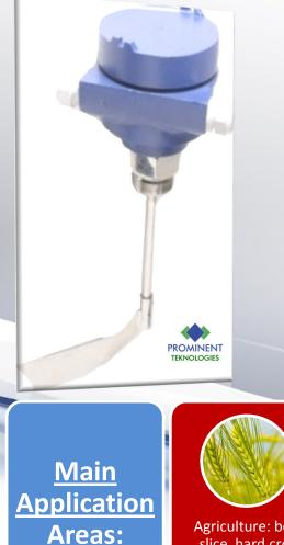
A small electric motor drives the paddle, which rotates freely in the absence of material. Impeded by material the motor will be turned within the housing while loading a spring and triggering two switches. One of them is a dry electric contact for control and alarm functions while the other cuts the power to the motor. When the material level drops, the loaded stretched tension spring returns the motor to its original position and the unit is reactivated.
